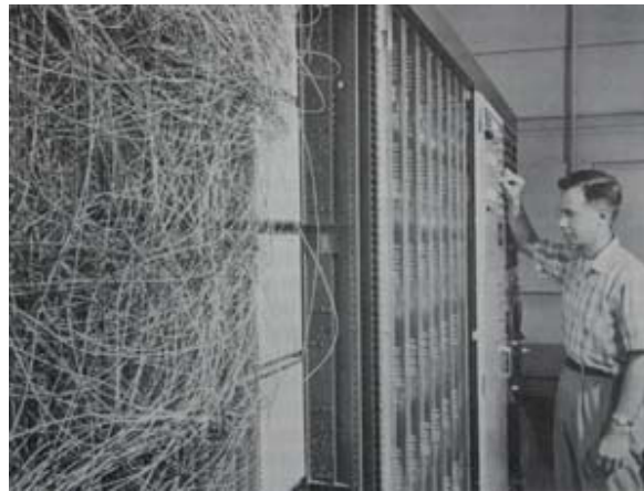
Patch board allowing configuration of inputs \phi
